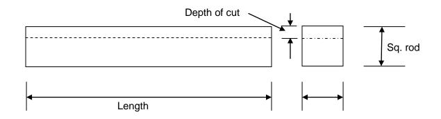
Module (M) = 1.5 Pitch =  $M \times \pi$ Depth = 2.157 x M Size of square rod =  $\frac{1}{2}$  x  $\frac{1}{2}$
