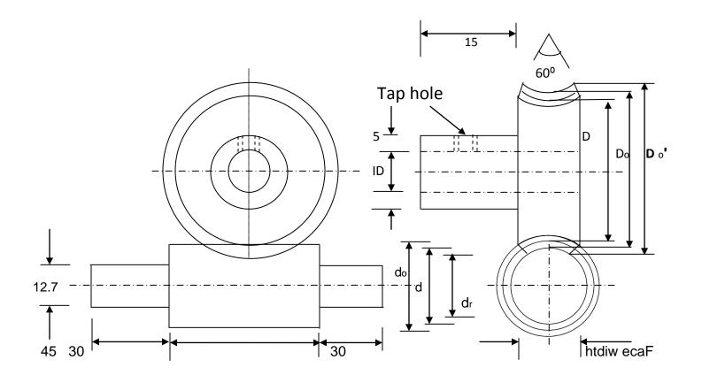
Ratio of Worm & worm wheel 1: 20 1:40 or Outer diameter of worm (do) 22 = Pitch of the worm 4.7 Depth of the worm Diameter over sharp corner (worm wheel) Do' Throat Diameter of worm wheel (Do) Depth of cut of the worm wheel Nos. of teeth of worm wheel = Gashing Angle (for milling m/c.) Face width of worm wheel Rod diameter (ID) 12.7 or 16 5.2 mm drill & ¼" tapping Tap hole size = Indexing for teeth cutting 40/N
